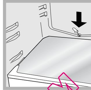
The refrigerator has an automatic defrosting function: water is ducted to the back of the appliance by a special discharge outlet (*see diagram*) where the heat produced by the compressor causes it to evaporate. It is necessary to clean the
