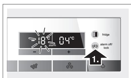
The temperature display indicates for 10 seconds the warmest temperature which was reached in the freezer compartment. Then the set temperature is displayed again.
