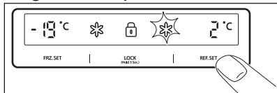
For temperature setting push **REF. SET** button until desired temperature displays.
