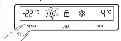
For temperature setting push **FRZ. SET** button until desired temperature displays.
