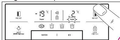
For temperature setting push **REF. SET** button until desired value displays.
