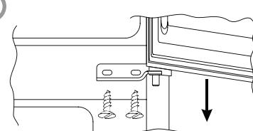
Remove the caps (A) and (B), loosen the screws and partially remove the panel.
