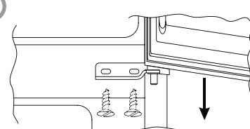
Retire as tampas (A) e (B), desaperte os parafusos e remova parcialmente o painel.
