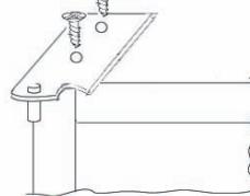
Remove the plug on the left-hand side and insert it on the right hand-side of the central and lower inserts.
