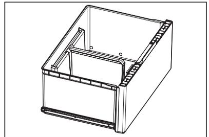
To regulate the humidity in the vegetable drawer the glass shelf incorporates a device with slits (adjustable by means of a sliding lever).
