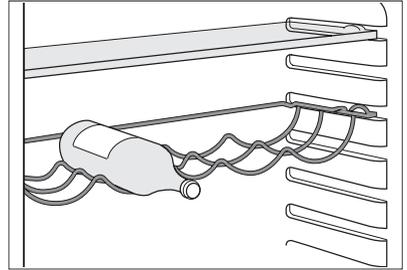
This bottle holder shelf can be tilted in order to store previously opened bottles. To obtain this result, pull the shelf up so it can rotate upwards and be placed on the next higher level.
